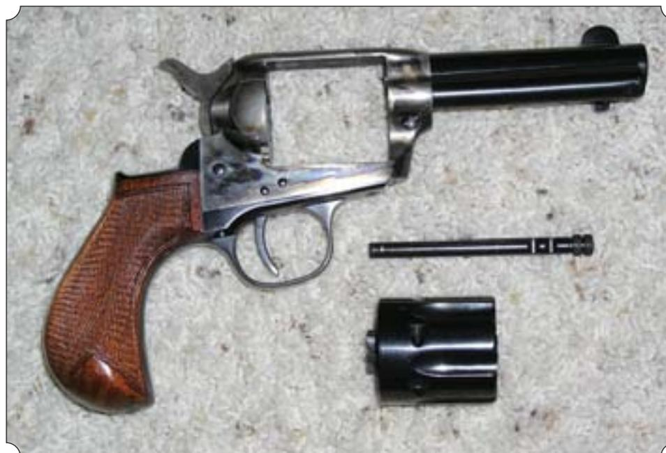
*The CIMARRON disassembled for cleaning. Note the two notches on the Base Pin. When pushed all the way in, the safety is engaged. When pulled out to the second notch, it's in the firing position.*
