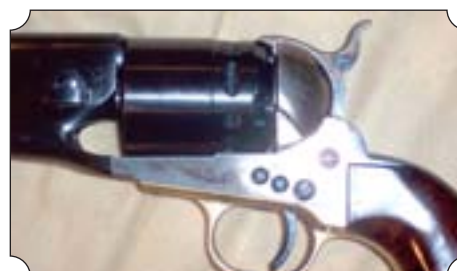
Close up of R&D's ten-stop cylinder design allowing this 5 shot revolver to be SASS legal.
