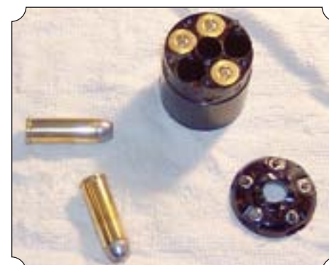
Rear face of R&D cylinder removed for loading in .45 Colt or .45 Schofield cartridges.
