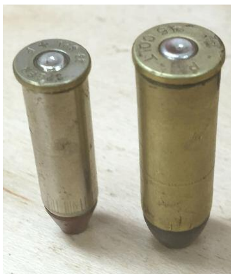
Fig. 1—Both the .38 and .45LC rounds shown here had good primer hits but were ejected from their rifles without detonating. Both had high primers.
