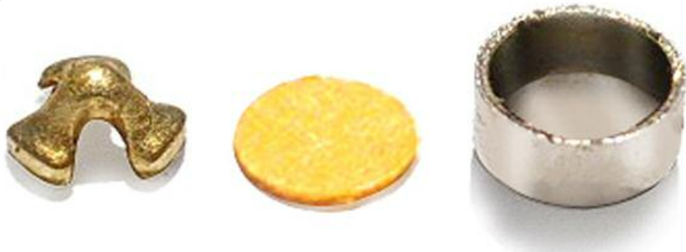
Fig. 4—The primer is comprised of three parts: a pyramid-shaped anvil, a highly explosive wafer, and the cap into which the anvil and wafer are fitted.
