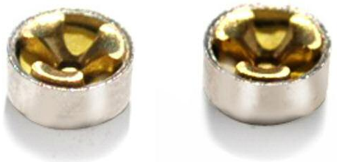
Fig. 6—The anvil in the new CCI primer on the left protrudes from the base of the primer by .010" for an overall height of .119". Once the primer has been installed in a case and compressed (right), the anvil gets squeezed into the cap about .005" but the anvil still protrudes from the base of the primer. (Look carefully at the two primers, the primer on the right has its anvil set slightly lower into the cap.)
