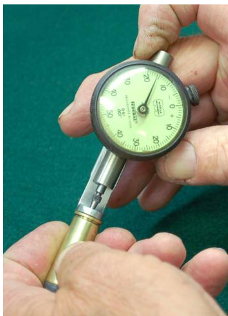
Fig. 2—Primer hits can be measured with a dial micrometer fitted with a special base that measures the depth of the primer's hit below the face of the primer. This primer hit measured .016"
