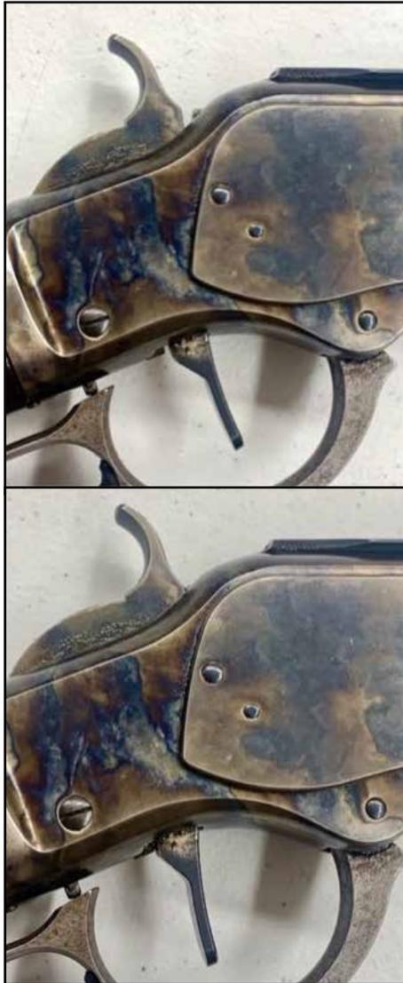
1860 HENRYS, 1866 AND 1873 WINCHESTERS HAVE A "SAFETY" POSITION WITH THE HAMMER JUST SHORT OF HAMMER DOWN (TOP). MAKE SURE THE HAMMER IS FULLY DOWN BEFORE TAKING A STEP AWAY FROM THE LOADING TABLE (BOTTOM).
