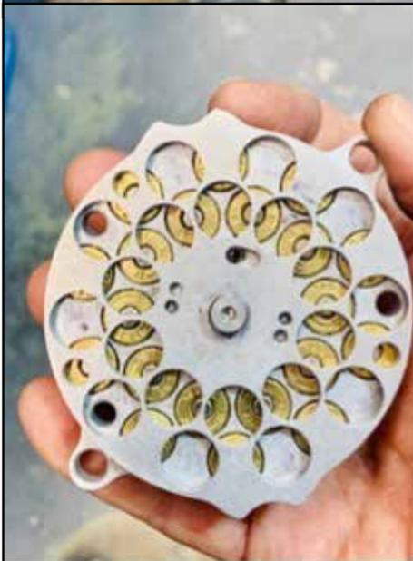
ST MACHINING LOADING BLOCK, OPEN. IF THE ROUND GOES ALL THE WAY IN SMOOTHLY AND WITHOUT RESISTANCE, IT HAS A GOOD CRIMP, A FLAT RIM, AND NO SPLITS. THE ONLY THING IT WON'T CATCH IS A CANNELLURE, WHICH CAN CAUSE A CASE SEPARATION, LOCKING UP YOUR RIFLE. CLOSING IT CHECKS ROUNDS FOR HIGH PRIMERS. MERNICKLE HOLSTER'S MAKES A POUCH FOR THEM. I HAVE SEEN THEM WITH ANTLERS TIED TO ONE OF THE OUTSIDE HOLES, THEN HUNG FROM A GUN BELT.
