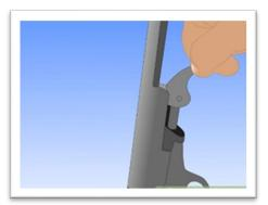
STEP 3: Seat the ball using the loading lever
