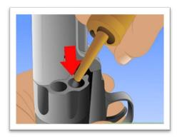
STEP 1: Pour a Measured charge (powder) into the chamber
