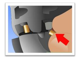
STEP 6: Place a percussion cap on each loaded chamber
