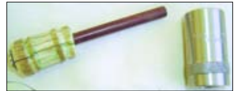
A Dillon Case Gauge for .38 Special, Part Number C32-15159, and pusher stick made from old ramrod and piece of antler carved for knob to expel tight or stuck cases. Also doubles as pusher stick when loading lever action rifles (saves the wife's fingernails)
