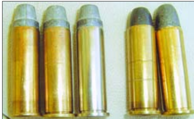
The three cartridges on the left are of different case design. Far left shows a case without a relief groove next to the rim. Next is a case with a groove that is shallow compared to the nicked case just to its right. The two cartridges to the far right show an uncrimped case with a bullet without crimping groove and 'sharp' case mouth edge and a Winchester factory cartridge that is smooth edged.
