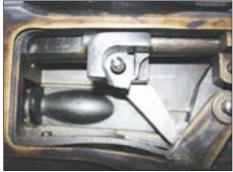
The major difference between the Uberti '73 and the Original Winchester 1873 is the use of the mechanical firing pin retractor and one piece firing pin in the Winchester. Shown is the firing pin retractor in a 3rd Model Winchester.
