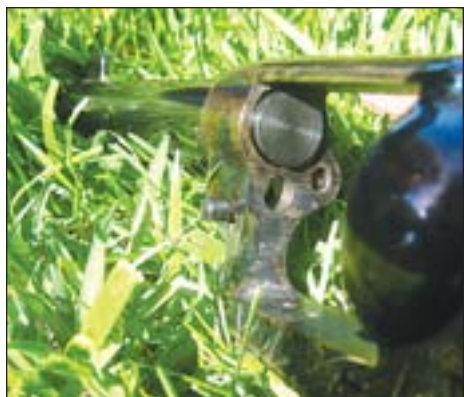
The barrel is permanently affixed to the frame and plugged at the base.
