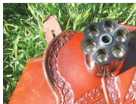
Cylinder holes are drilled to a depth of 9/16th of an inch from the back and 1/2 inch from the front end.
