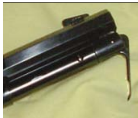
Takedown starts by using the supplied lever and unscrewing the magazine tube.
