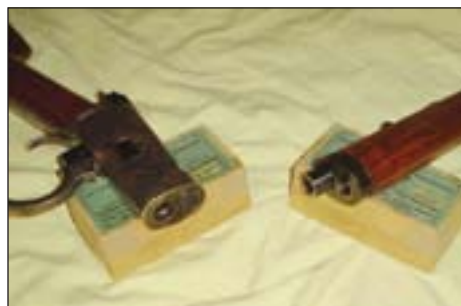
After removing the magazine tube, a final 90-degree twist frees the barrel from the receiver. Breaking the rifle down into two major pieces allows easier transporting as well as facilitates cleaning (especially blackpowder cleaning!).
