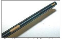
Cartridges are loaded directly into the magazine tube.
