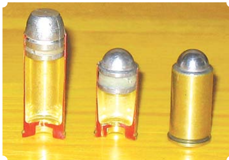
Shown here are two cutaway cartridges to help illustrate the change in case capacity. On the left is a .45 Colt with a 200 RNFP bullet and in the middle is the Cowboy .45 Special with a prototype "EPP UG .45-147 boolit" named by Dick Dastardly for it's original creator, El Paso Pete (deceased SASS member). Dick has the molds on order. On the right is a round loaded with the EPP UG .45-147 bullet.
