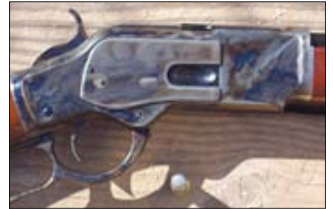
This sample had really exceptional color case hardening, considering it is chemically done. Original bone case hardening would make the cost prohibitive.
