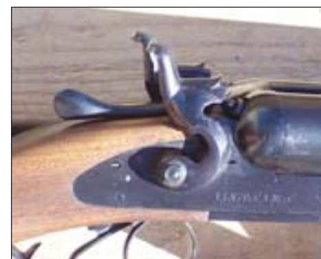
Check the hoods above the face of the hammer for sharp edges, and file if necessary. They can cut you when cocking both at once with the palm of your off hand.
