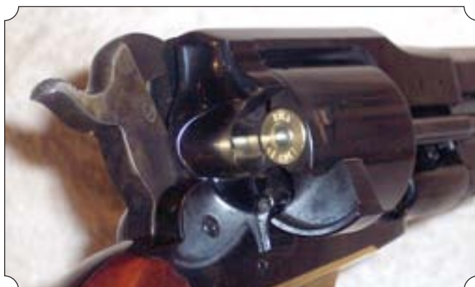
Close up of the 1858 Conversion's loading gate.
