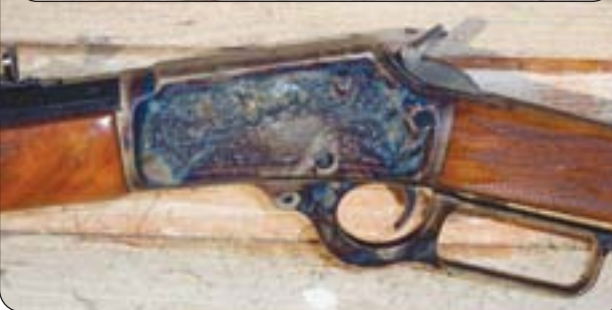
Beautiful Doug Turnbull real bone color case hardening on the Century Limited's receiver.
