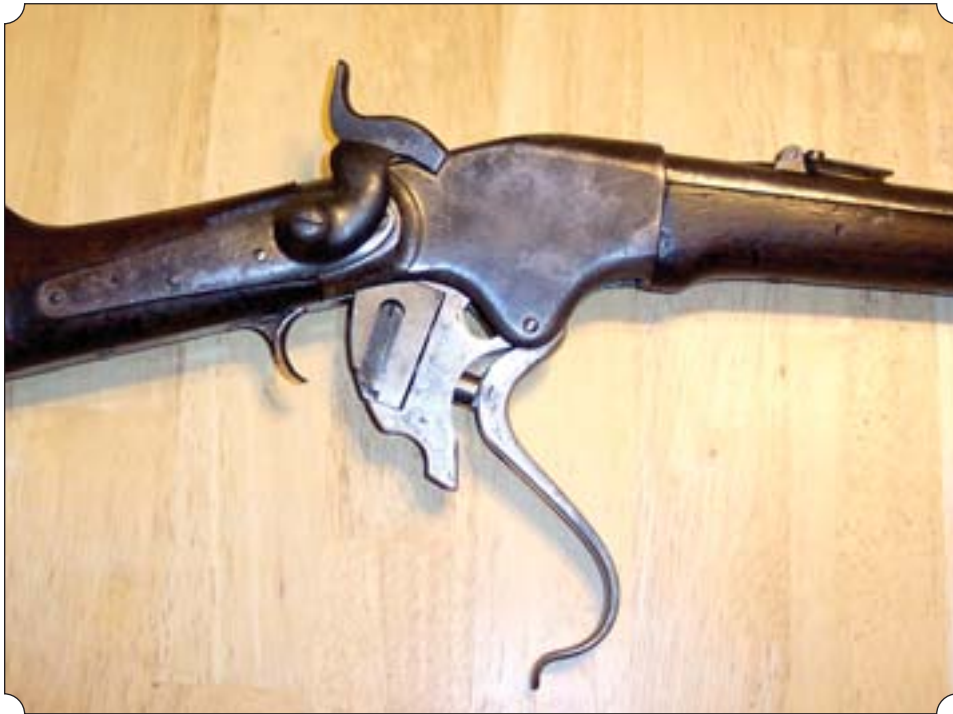
Spencer lever is pulled down to open action and allow a round to enter action from chamber.
