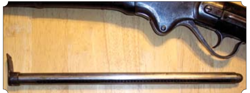
Magazine tube that holds seven rounds in the Spencer stock. Works like magazine in stock of early Browning semi-auto .22 rifles.
