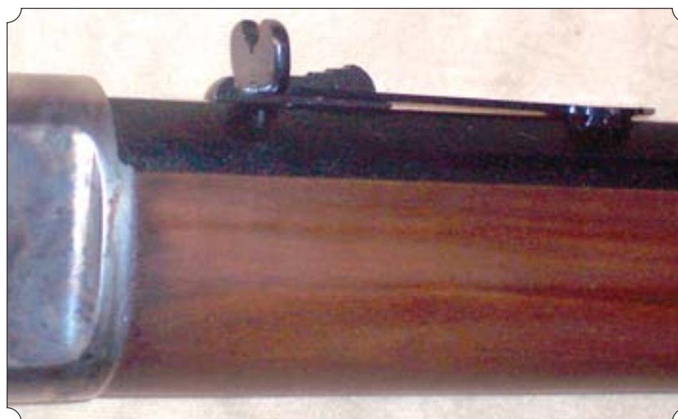
EMF's Winchester 1892 has a close copy of the original Winchester rear sight, rather than the stamped metal one of other 1892 replicas.
