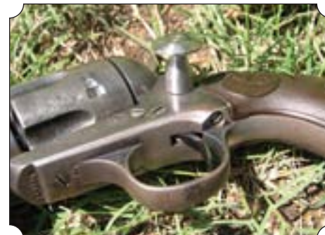
This is the special hammer stud shown installed in a first generation Colt SAA.
