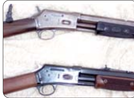
The heart of every Lightning's action is the pump.
