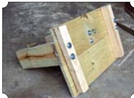
Photo 1: Back wall and axel support assembly. Note the notch cut at the upper left hand corner. Note how the corner braces are set in 5/8" and are 5/8" from the bottom to accommodate the mounting of the sides and bottom.
