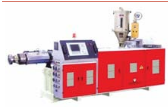
Extrusion machines produce long continuous shaped products such as tubing, gutters, lawn trim, and down spouts.
