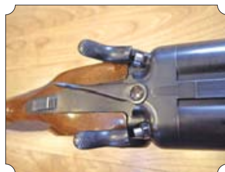
The hammers have hand-cut knurling, no sharp edges, and light springs.
