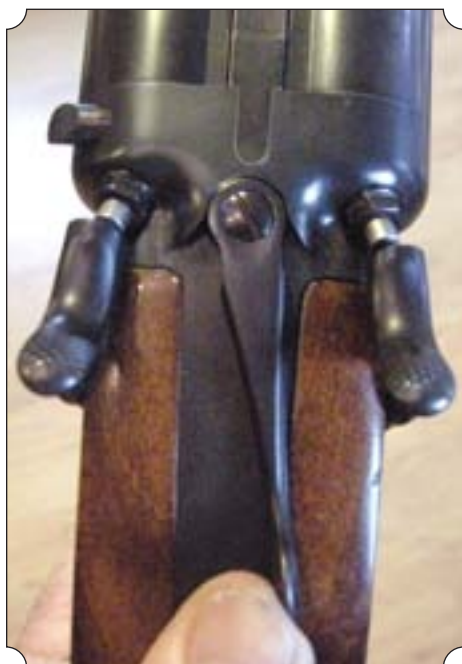
The operation of the Greener action: The lever is pushed slightly, and the cross-bolt is moving to the left to release the barrel lock.
