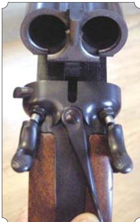
As the lever is pushed further, the cross-bolt releases the barrel lock, and the barrels open, extending the extractors.
