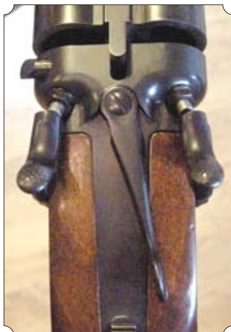
Pushing the barrels upward extends the cross-bolt, allowing the barrel lock to align with the cross-bolt, locking the barrels closed.
