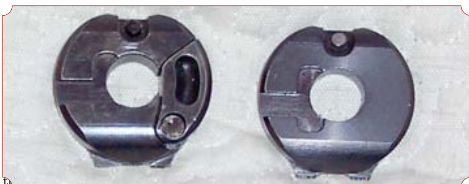
Current gated Konverter ring (l) and early non-gated ring (r).
