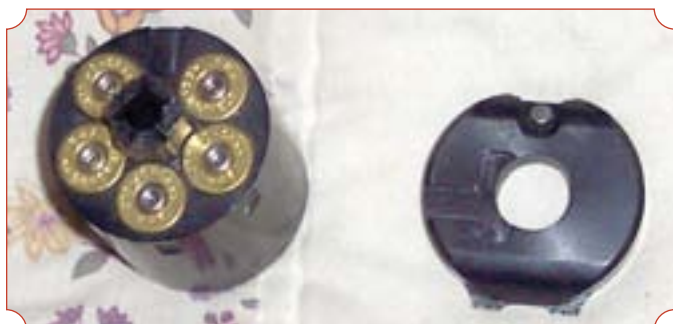
Two piece Kirst Converter with five .45 Schofield cases in the chambers. The sub-caliber "Safety Chamber" is really more of an empty slot for the hammer/firing pin to rest in. Note the single firing pin in the recoil shield and two small feet on the bottom to eliminate excess movement of the recoil plate.
