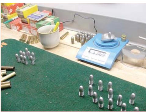
By weighing each cast bullet, the shooter can weed out ones that are out of spec weight-wise. For real precise shooting, plus or minus a couple grains is okay, but serious long range shooters won't compete with a bullet that is off by more than .2 grains!
