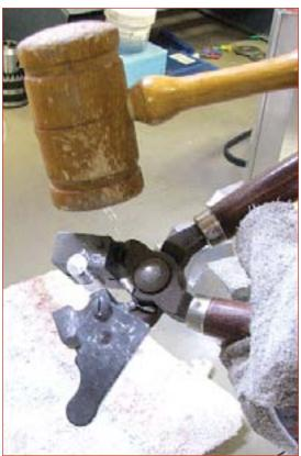
Tapping out the bullet with a piece of wood or mallet onto a cloth ... the bullets are soft, and a towel or other soft landing keeps them from denting.
