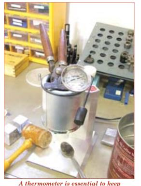
the lead around 800 degrees. The alloy stays together, and the lead flows and cools the best at this temp.
