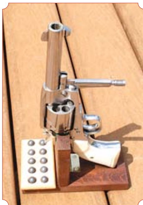
A Revolver Loading Stand (Dixie Gun Works) gives you another hand or two. This one has been improved with a 10-round ball holder.
