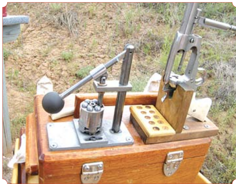
Capt. Baylor's setup includes a separate cylinder loader. This one from Powder, Inc. is the best currently available.
