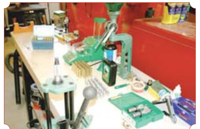
I like my table organized for loading black powder so no other components can be mixed in by mistake. The RCBS large loading press is better for the long cases. Some of the other presses don't have enough free throw, and the case and bullet have to be angled into the press and die to be seated.
