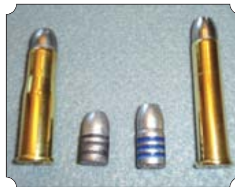
.45-75 cartridge and bullet compared with .45-70.
