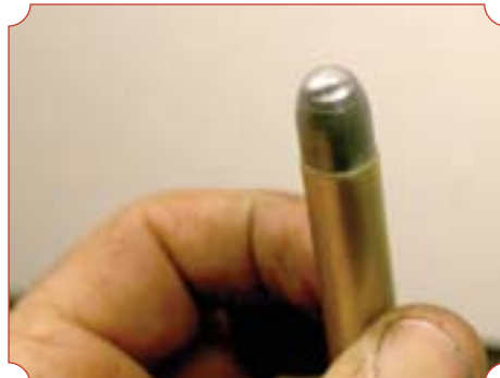
The soft lead of the 20-1 alloy will dent if it is not straight in the sizer. Also, the nose will deform if too much compression is attempted.
