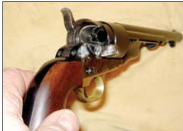
Author's Pietta after cutting cartridge loading channel with Kirst Konverter.
