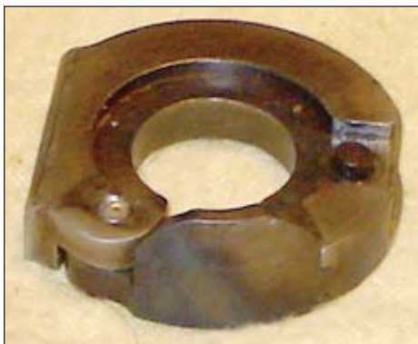
Color case hardened Konverter ring can be used on either standard or modified 1860 percussion revolvers.
