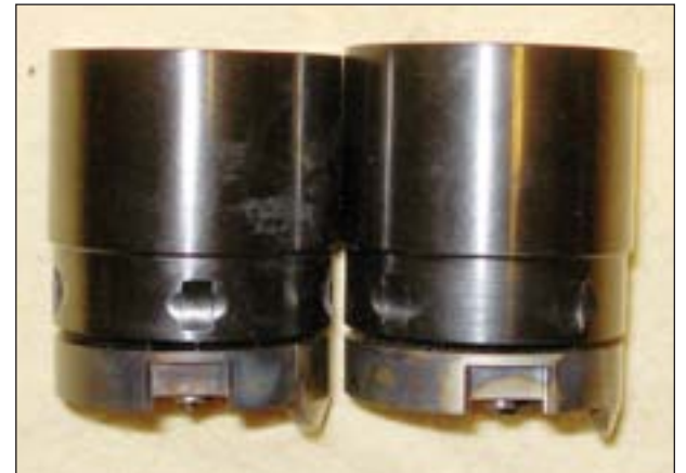
Photo shows the Konverter unit. Shorter one on left is for Uberti 1860, and the longer one on right is for Pietta.
