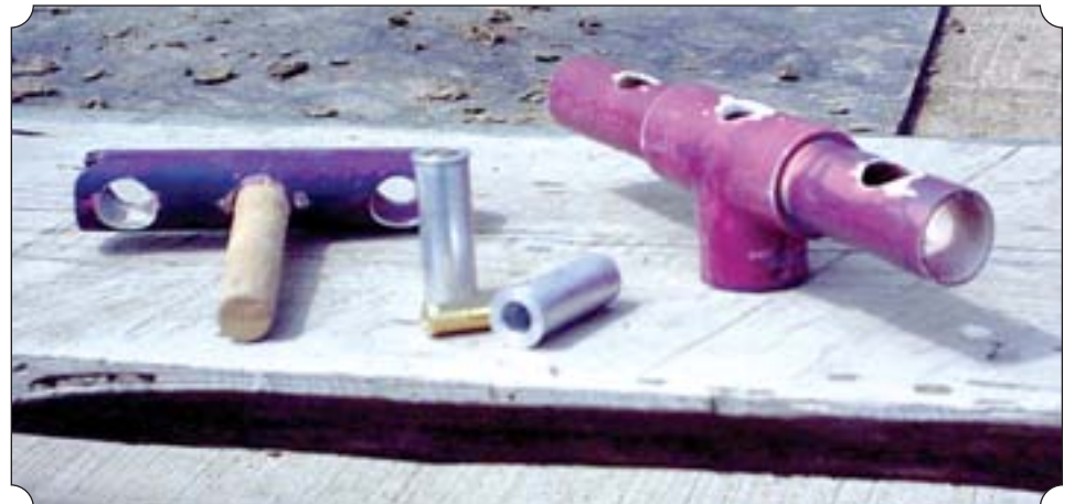
The special .45 caliber shotgun inserts are seen in the middle, and the two special balloon holders are seen on either side.
