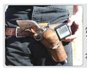
High tech helps ensure cross draw holsters are "safe." Cross draw holsters must not be canted more than 30°; however, quickly testing for unsafe holsters on the Range has always been a challenge. An electronic protractor was used at Winter Range to make a few quick checks and challenge a couple of offenders. END of TRAIL has just purchased three. There's no arguing with "high tech!"
