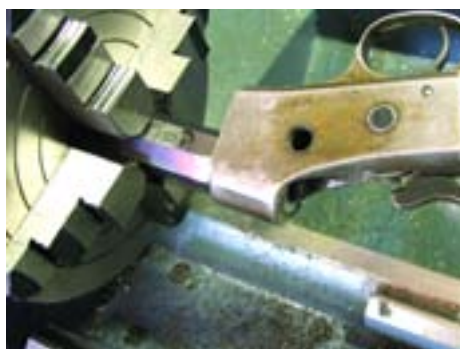
Checking the fit – The first step was to barrel the action with a .45 caliber barrel. A nice tight Class 3 fit was what I was after. This involved taking off a couple thousands and trying it. After numerous tries, the fit was perfect.
