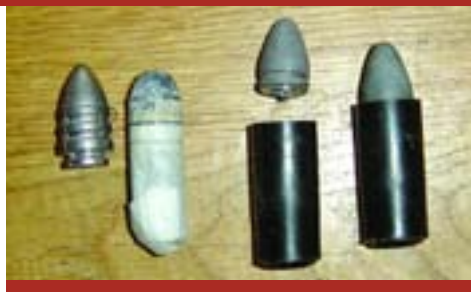
Sharps paper cartridge on (left) and Smith rubber cartridge on (right).
