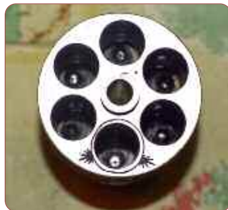
Frontiersmen want to be able to leave the same chamber unloaded every time. On the outside I had Aspen Filly engrave the last 3 digits of the serial number over the correct chamber. On the front of the cylinder, Aspen Filly engraved this circle with emphasis marks so I can keep it empty.
