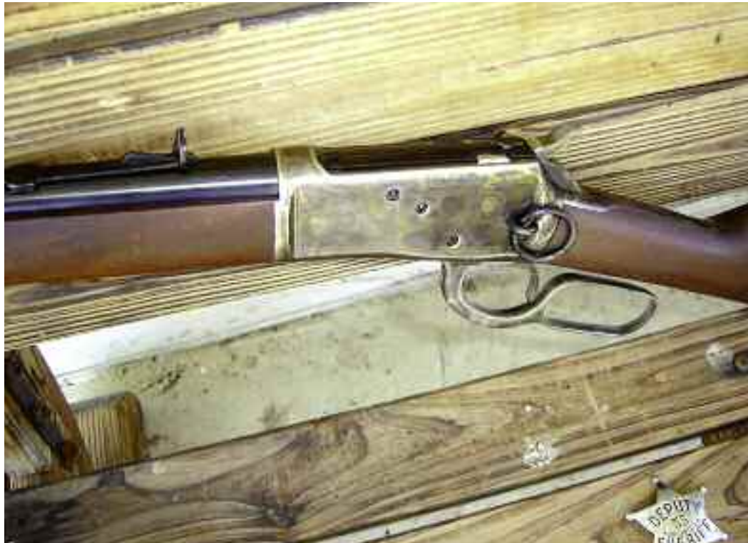
Well done Winchester style rear sight, saddle ring, and color case hardening.
