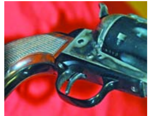
Smokewagon trigger is standard Colt SAA trigger, narrow, and offset to the left
