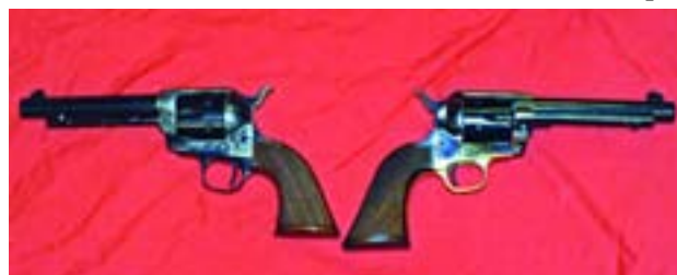
Taylor's and Co. Smokewagon on the left with SAA grip frame and the Alchimista on the right with the 1860 Army grip frame
