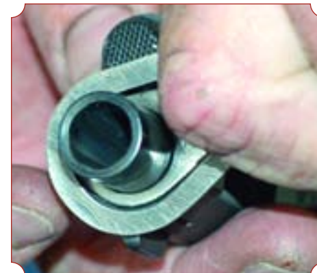
The Screw Wrench at work on a 1911.
