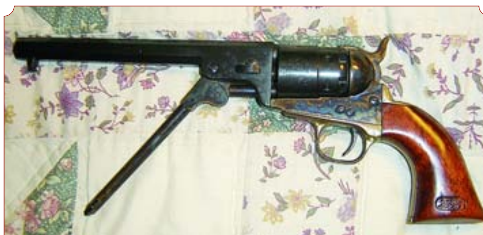
The loading lever is used to ram the balls on top of the powder charge. Note the nice inspector cartouches on the pistol grip of the Hartford Model.
