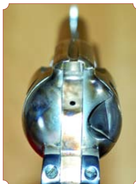
Cimarron Evil Roy hammer for comparison, standard height. Wide rear sight slot, wide front sight.
