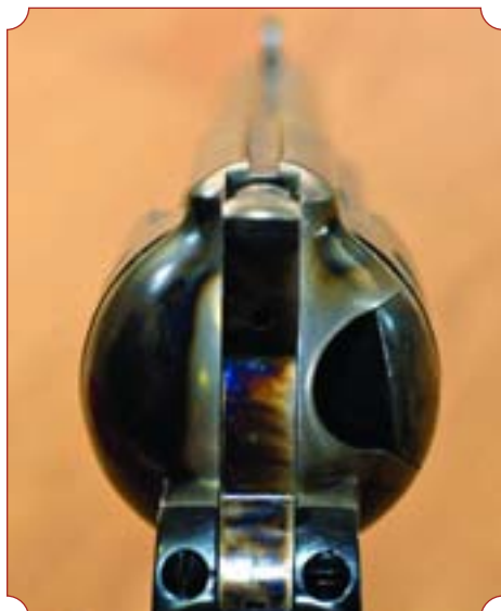
The "Stage Coach" hammer is .10 in. lower than stock Uberti hammers. Note wide rear sight slot, wide front sight.
