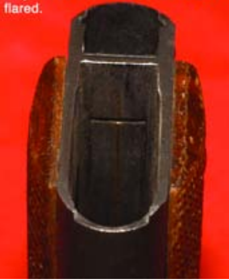
Colt's beveled mag well. Beveled mag wells are allowed in both categories.
