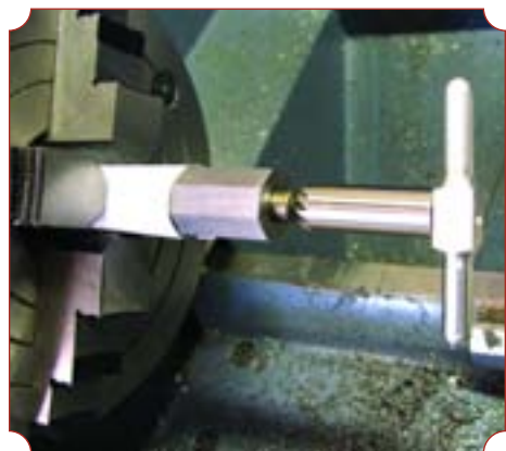
Crowning the muzzle protects the end of the bore, ensuring the end of the bore remains absolutely perpendicular to the centerline.
