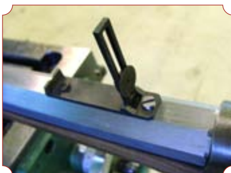
The rear sight is a Rough and Ready vintage-style sight bolted to the top of the barrel.
