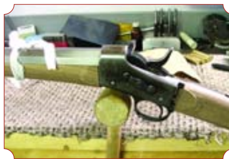
The forearm grip required fitting as well. Drilling and threading the needed attaching hole and glass bedding completed the effort.
