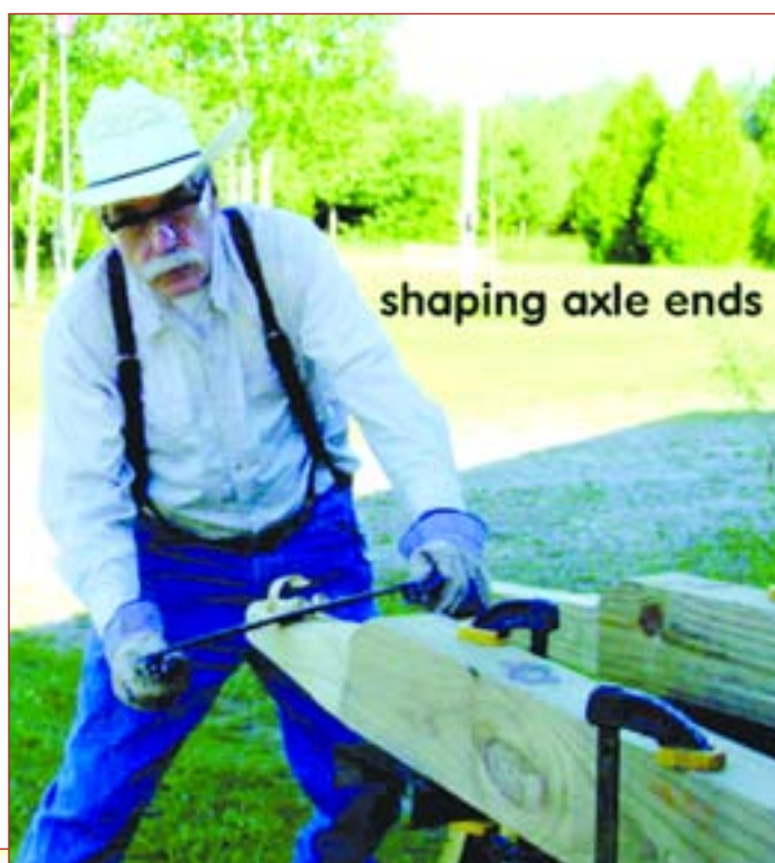
copying original axle taper
