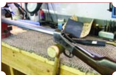
Before getting too deep in the project, it's always a good idea to make sure everything is going to work. Mating the barrel, receiver, and the original stock provided the necessary foundation for testing.
