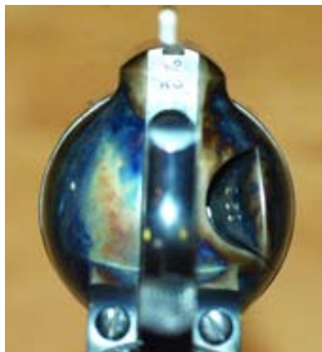
Wide front sight and .140" wide rear sight notch makes quick acquisition of the sight picture easier.
