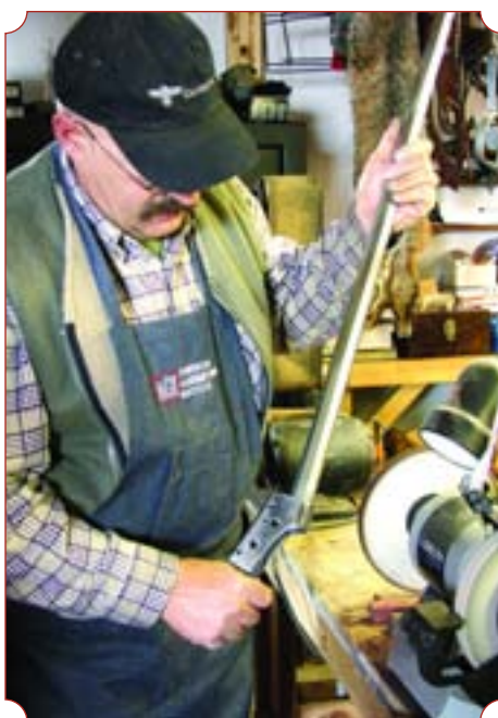
Polishing the metal is a progressive process, but once the pits and scratches are all out, the finished product is beautiful.
