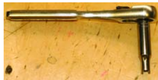
1/4" drive 3/16" deep socket modified to fit Treso nipples perfectly by Larsen E. Pettifogger (not for sale).
