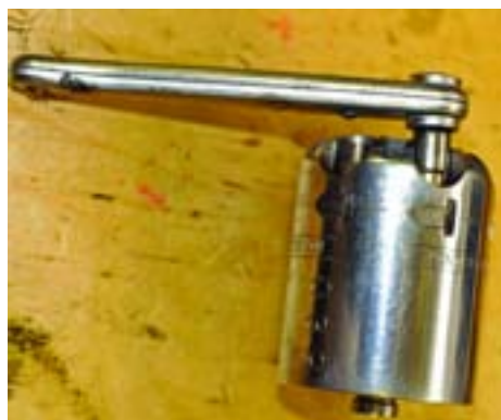
The ratcheting nipple wrench from The Possible Shop. It is cut to fit Treso nipples perfectly.
