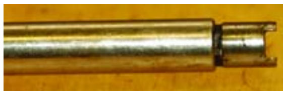
The socket from the Possible Shop's ratcheting nipple wrench in a Brownell's Magna Tip® Screwdriver handle (part #080-087-000).
