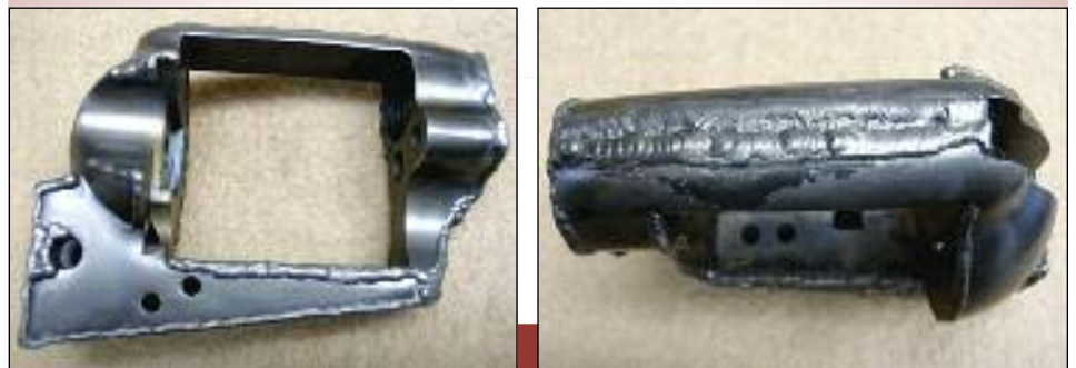
The first step was to add metal to the frame so it could be re-profiled to original dimensions.
