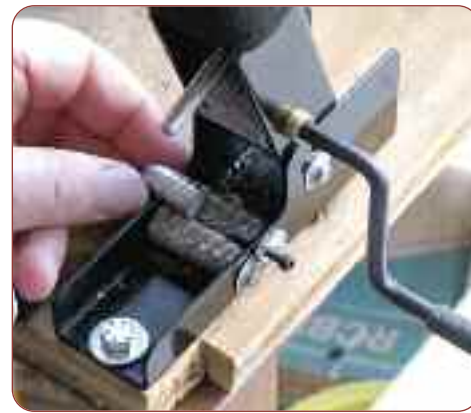
Details of the knurling machine. One complete turn of the handle and the driving bands are textured to hold additional lube.
