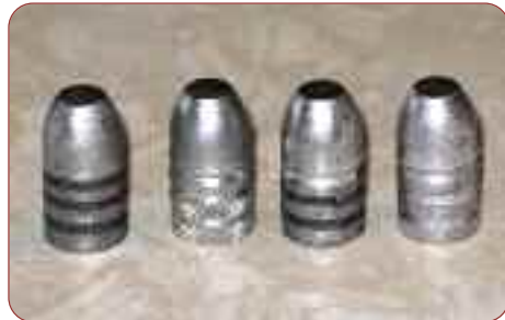
From right side—an as-cast 340 grain bullet for the .45-75. Next is the bullet with regular sizelube. Third is a cast bullet after knurling, and fourth is that bullet after sizing and lubing. You can see the small indentations with lube embedded into the driving bands to add much more lubricity.
