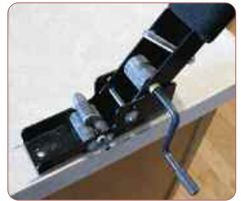
Details of the knurling machine. One complete turn of the handle and the driving bands are textured to hold additional lube.
