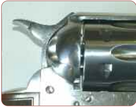
The Super Blackhawk-style lowered hammer on the Runnin' Iron
