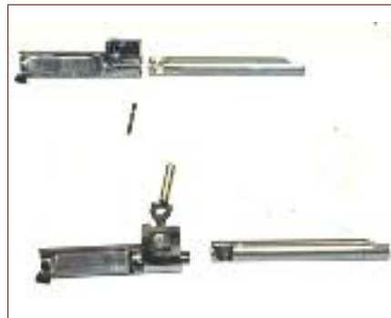
The old (top) and new bolts are shown disassembled. The beefier pin retaining the bolt extension is obviously much stronger and offers considerable peace of mind.
