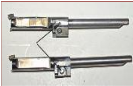
Old Uberti '73 bolt on top. Note the small pin. That holds the bolt and bolt extension together. New Uberti '73 bolt on bottom. The small pin is missing. That BIG cross pin holds the bolt and bolt extension together.
