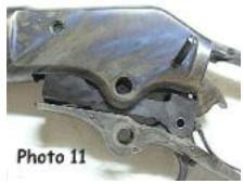
another interesting feature of the Burgess. The hammer screw shown in Photo 11 goes through the hammer, but it does not actually retain the hammer. The hammer and the carrier both pivot around the little tube shown just above the trigger in Photo 11. The hammer screw goes through this tube.
