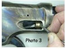
held in the magazine by the stop. Looking down into the ejection port, we can see a cartridge being held by a split carrier that grips the cartridge and holds it in place for insertion into the chamber. Photo 4.
