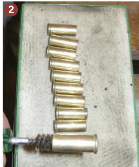
Brush cleaning inside of case and cases on a lubrication pad.
