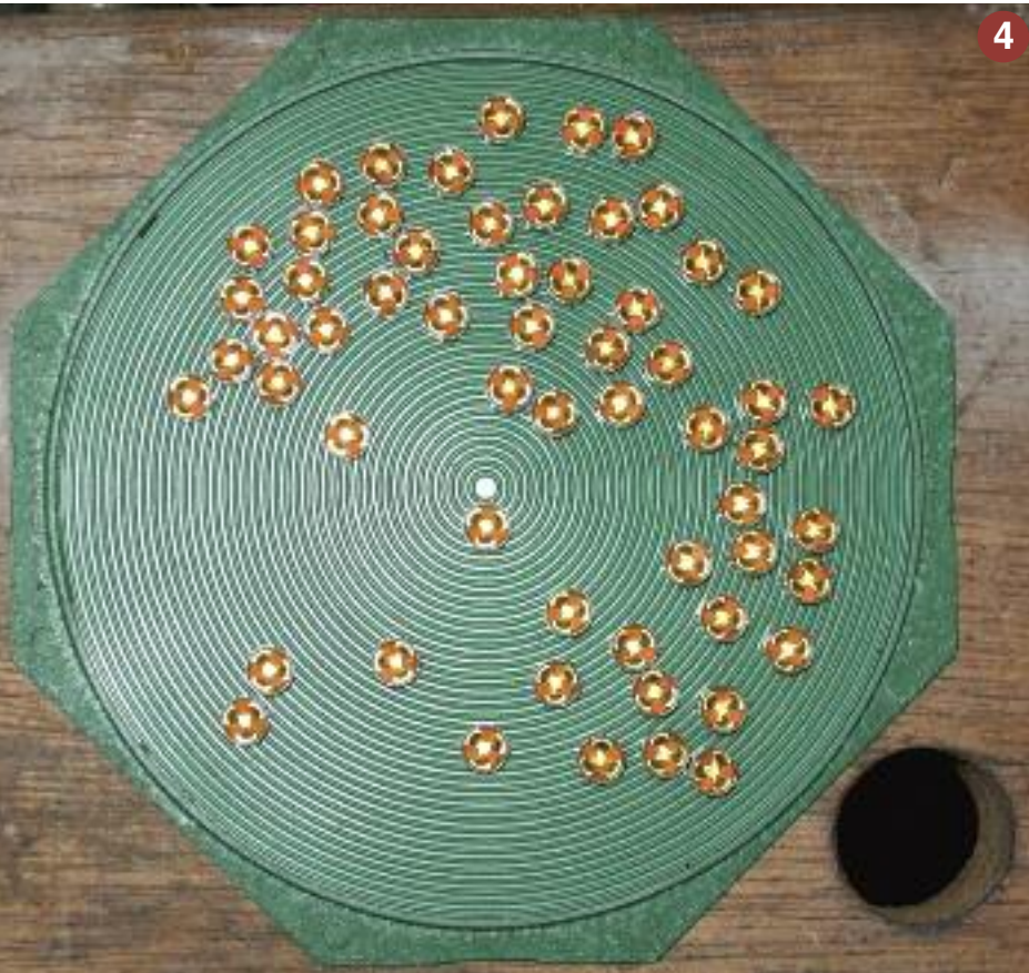
Primers on the primer tray after the tray has been rotated in a circular fashion to get all primers facing in the upward position.
