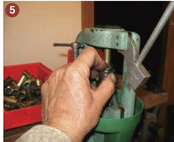
Priming - Index finger keeps pressure against the case and shell holder while the thumb presses the primer arm into the slot for priming. Also note the primer tube is shown in this figure.
