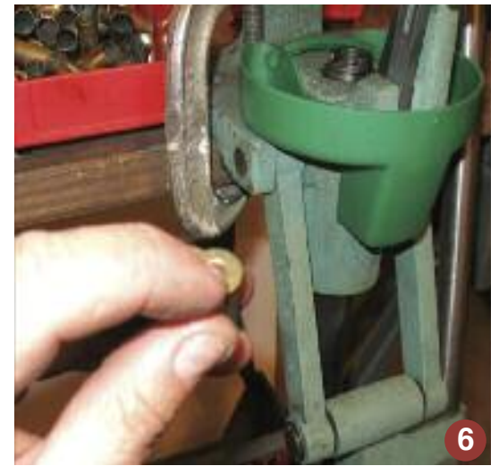
Checking for high primers by running your index finger along the case head and primer.
