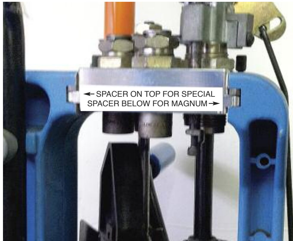
With the laser cut steel spacer on top, the tool head is set up for .38 Specials. With the laser cut steel spacer on bottom, the tool head is set up for .357 Magnums.
