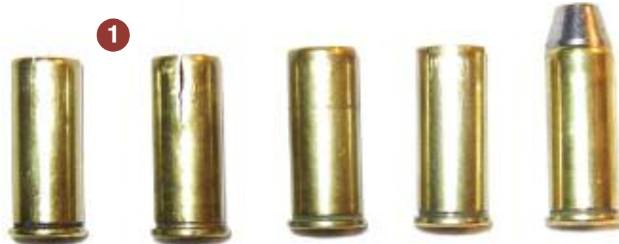
From left to right—A slightly ruptured case to discard; a severely ruptured case to discard; a fired case with rolled crimp that is not resized, note the slight mouth constriction; a correctly resized case, note the expanded or flared bell shaped mouth opening; and a completed cartridge with bullet and crimp.
