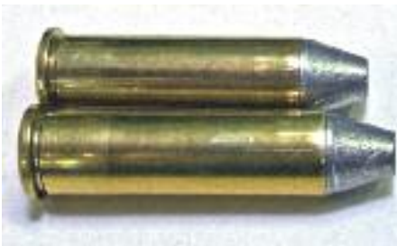
Sample .38 Special and .357 Magnum rounds loaded with the adjustable tool head
