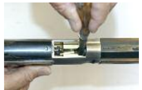
Insert the screw knife tip into the carrier in between the two rounds and ...
