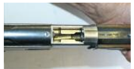
"The '66-'73 jam." Usually a split case allows the bullet to retract into the case, making the overall length too short and locking up the gun. The next round slid halfway into the carrier preventing its lifting.
