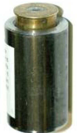
This round failed, sticking at the point shown. It might not chamber or extract easily in competition.
