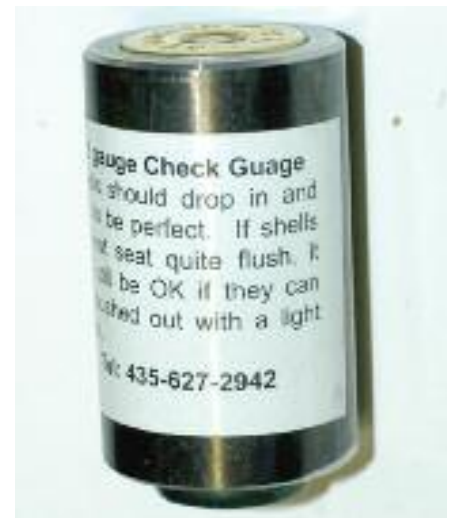
12 Gauge Check Gauge with a round that passes.
