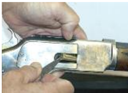
Extract the bad round from the loading gate. Sometimes the rounds pop out easily. Sometimes pushing the round forward with the screw knife and releasing will allow it to pop out. Then work the lever to load the next round. FRONT SIGHT! Resume firing. Remember to load a fresh round to replace the bad round.
