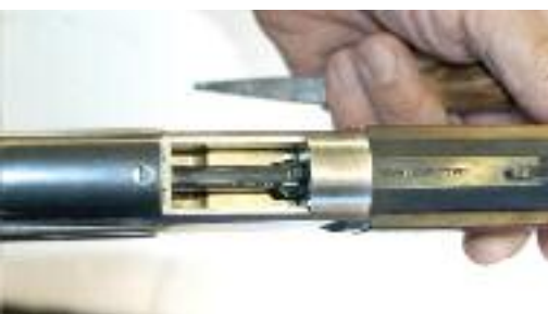
Close the bolt, sliding the knife out as you do so.
