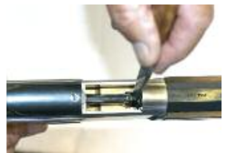
... push the "next" round toward the muzzle until it is in the magazine tube again, freeing the action.
