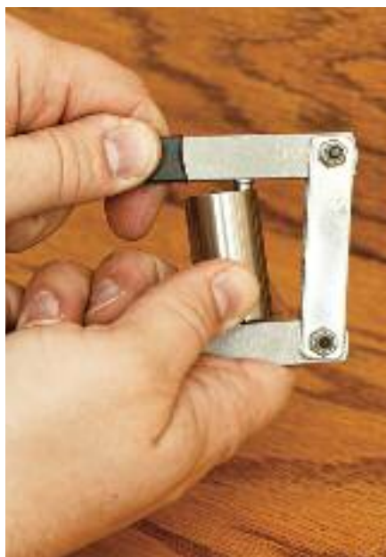
Since none of these percussion revolvers have an integrally mounted ram, the cylinder must be removed and a manual press employed to seat the bullets.
