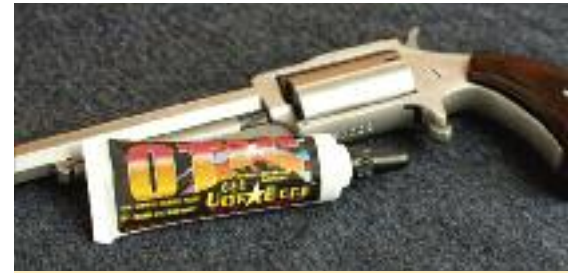
A few drops of Otis Ultra Bore on the frame-mounted firing pin every 15 shots or so kept everything well lubricated and working.
