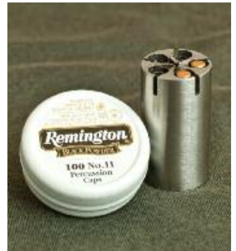
Tolerances are tight on these revolvers! Remington #11 caps reliably seated snug and out of the way, ensuring no "high-cap" binding as the cylinder turned.
