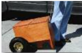
To move the cart on the ground in the stowed position, an aluminum handle is provided. Hook it in the front hasp where the lock would go, and you're ready to roll. The handle can be stored inside the cart as well.
