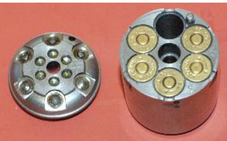
The backing plate next to the cylinder. Note the empty chamber is to the left of the locator pin.
