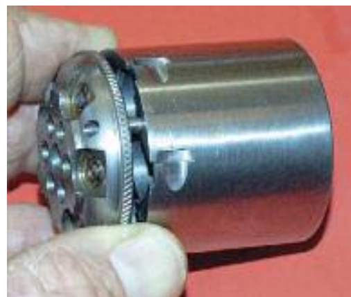
R & D Conversion Cylinder shown with backing plate pulled away to show the locator pin. This locks the backing plate into place.
