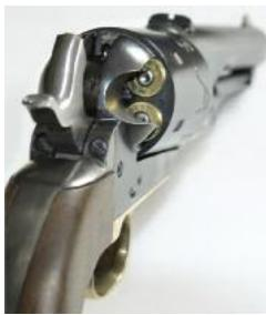
Like the originals, the Centaure Long Cylinder Conversion has no loading gate. That works fine as long as you are not cocking the pistol while aiming at the sun! Similar to the later Colt Open Top, a number of these Long Cylinder Conversions had their rear
