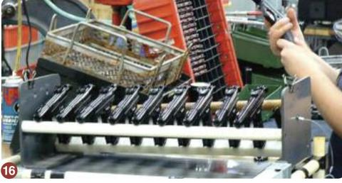
the parts for the blue, the stainless steel, and the polymer frame models are different. Yet because of Ruger innovations, they can all be assembled at the same time. **Photo 16** shows the tenth gun getting ready to be put into a ten-gun tote.
