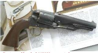
Centaure Marshal #12089 converted in 2010 by German gunsmith Klaus Mumme into a Long Cylinder Conversion chambered for .44 Colt. Note straight cylinder. Originals chambered for .44 Henry rimfire were probably made by gunsmiths in Mexico about the same time Colt manufactured their Thuer conversions during the late 1860s.
