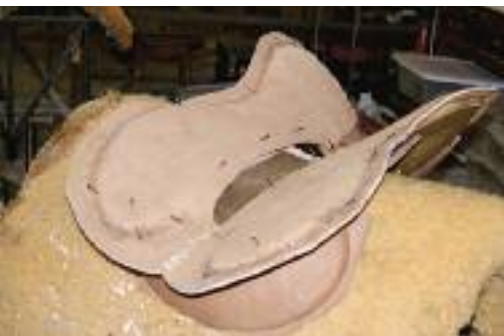
Photo #3. Skirting tacked to tree and molded to fit
