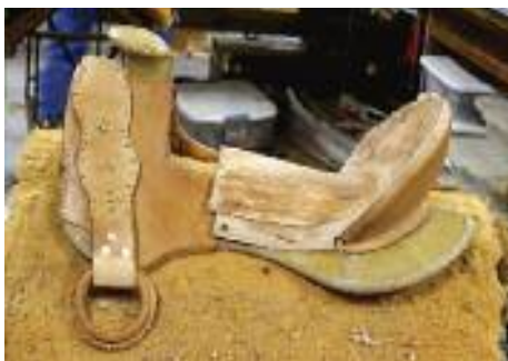
Photo #6. Fore-end rigging tacked in place
