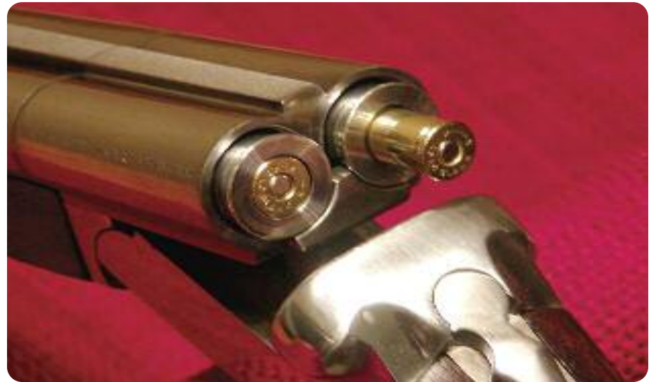
The inserts with the .45 caliber blanks are loaded in the shotgun just like normal 12 ga. shells.
