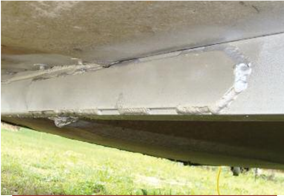
Channel welded to back with fish plate
