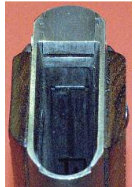
Gunsmith Wild Bodie Tom beveled this magazine well on a Colt, making speed reloads a little quicker. You still have to practice.
