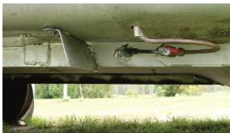
Channel installed and painted with stone-guard to protect gas line
