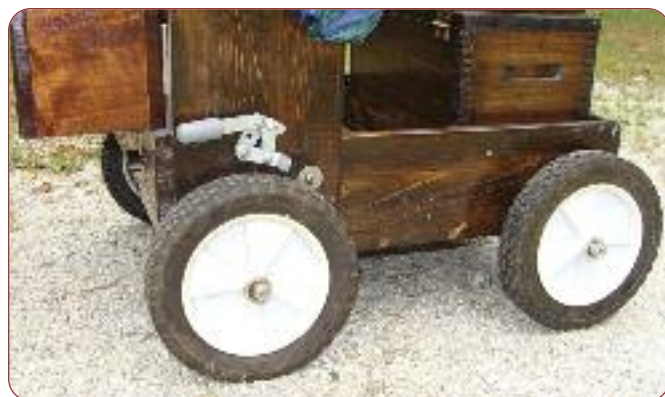
Cart wheel showing added braking system
