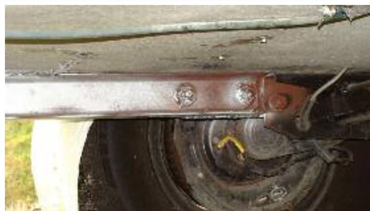
Channel bolted and welded to axel plate
