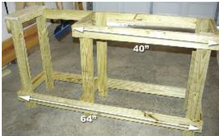
Loading table with legs attached to upper and lower frames. Lower frame is 3 1/2" from the ground (width of a 2x4). Note the "corral" area for the loading officer is on the left (but would be on the right for an unloading table).
