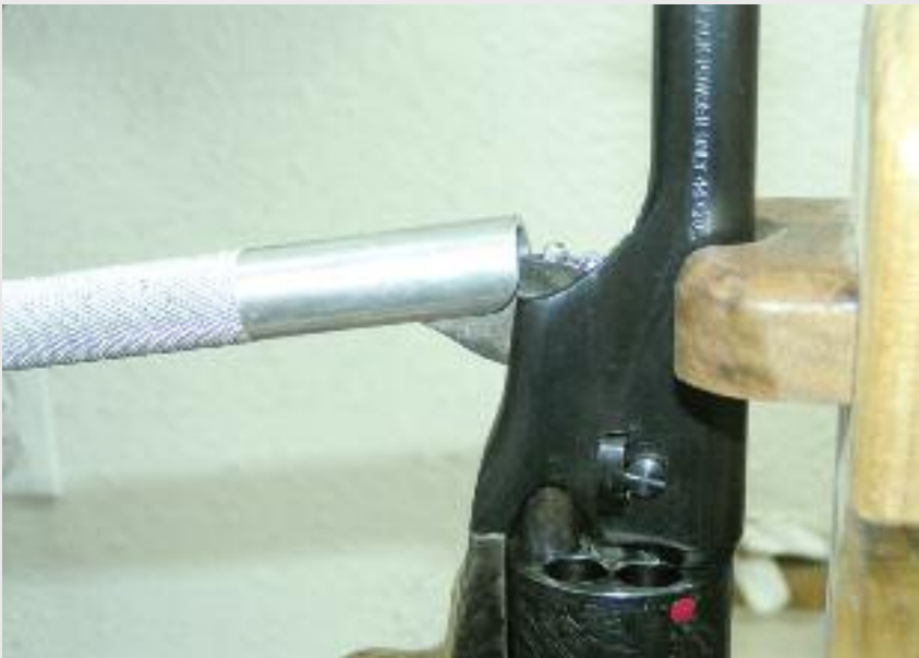
A standard SliX-Hand on a "X"-1/2" Colt. Notice the radius on the mouth of the hand has been modified to clear the frame with the shorter barrel and loading lever.
