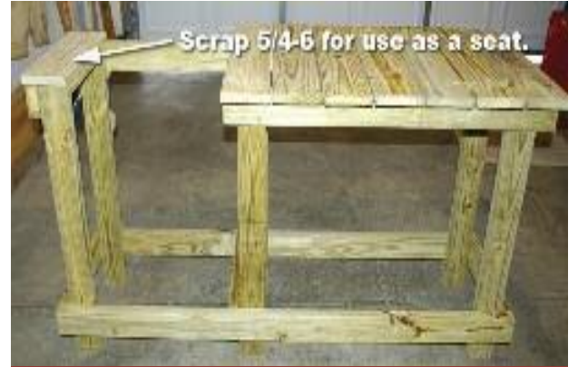
Loading table with top slats (5/4-6, 26" in length) attached.
