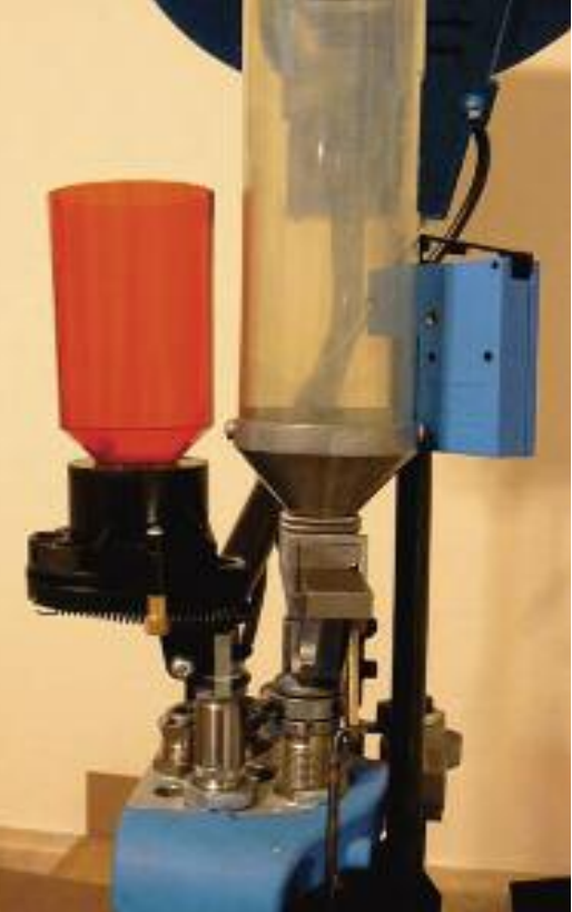
The Dillon powder measure dispenses powder. The Lee Auto Disk powder measure dispenses filler for wimpy (or arthritis friendly) loads for cartridges beginning with .4. (Larsen E. Pettifogger photo)
