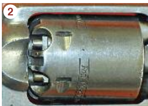
The SliX-Shot nipple is on the top. It is visibly longer than the Treso nipple on the bottom.
