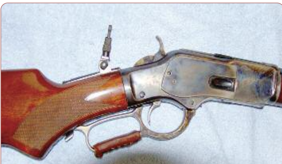
Side view of peep sight—The sights come in different angles to fit the angle of the rifle tang on which they are to be installed.
