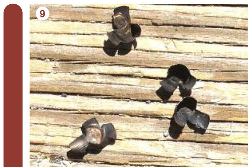
9 These four caps opened up and fell off when the cylinder was rotated at the unloading table. The fifth cap had not opened up and was easily pulled off. Both results are good.
