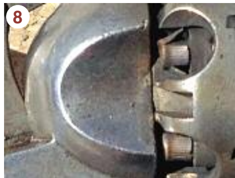
8 Fired caps. The upper cap has opened up on firing. This is desired as the fired cap will fall out and not jam the action. The lower cap has not opened up or fragmented at all. This is also desirable, even if the cap has to be pried off at the unloading table.
