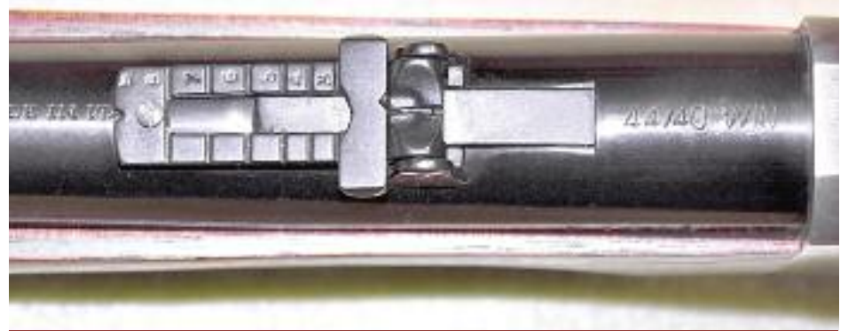
Rear sight on Spencer with Battle Sight notch deepened
