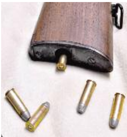
Spencer's tubular seven-shot magazine in the butt stock
