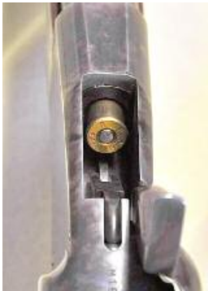
Spencer with .44-40 round single fed into top of receiver
