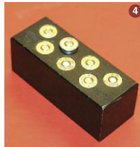
Photo 4—EGW Case Gauge for .45 ACP. Second round on the top has a bulged case
