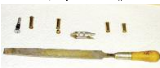
Fine mill file in foreground. Background L to R, mandrel, .38 Special brass case, trimmed case, deburring tool, and right two are trimmed and finished brass.
