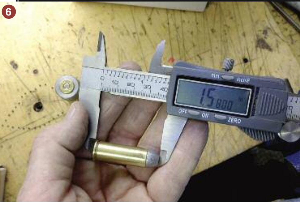
Photo 6— I've locked the caliper at 1.58. Any round that passes through will fit in my Uberti '73 made in the 1990s.
