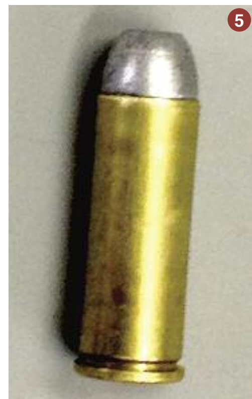
Photo 5—.45 Colt with 200 gr. LRNFP bullet correctly loaded, note roll crimp into the crimp groove
