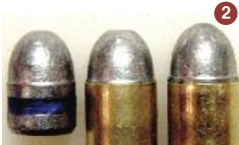
Photo 2—left to right: A 230 gr. LRN bullet, a round with the bullet correctly seated and crimped, a round with the bullet seated too long and the brass crimped into the lead.
