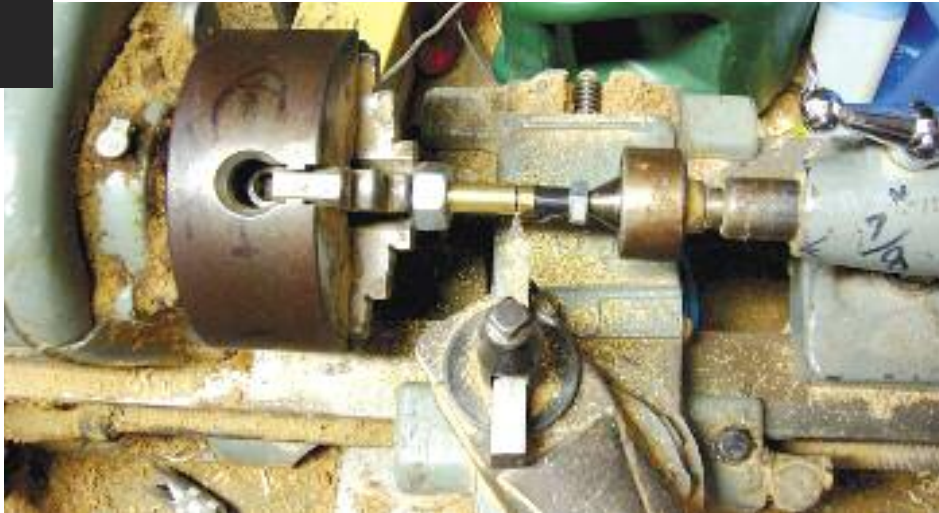
Small metal lathe set up for trimming brass.
