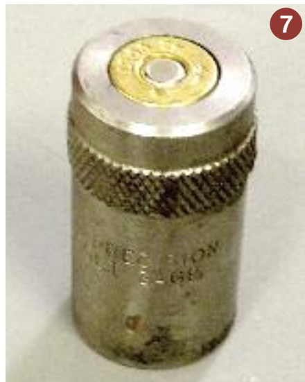
Photo 7— .45 Colt Chamber checker/case gauge with a round that passed inspection.
