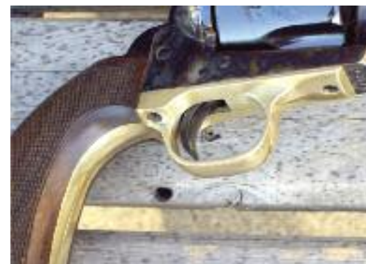
Wide, set back trigger leaves plenty of room inside the trigger guard for big fingers.
