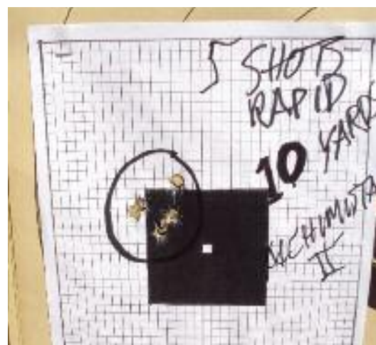
10 yard target shows this particular gun shoots slightly high and left, but tight groups are the norm—even with rapid fire!
