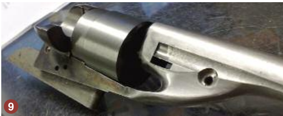
... and cylinder installed. Note slot on the right side of the barrel for the ejector housing
