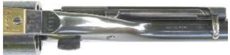
Proof marks, caliber stamp, and NK again for Karl Nedbal under barrel
