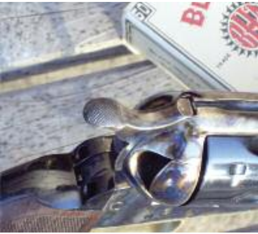
The wide hammer spur makes for fast action, and is dramatically easier to cock when shooting one-handed.
