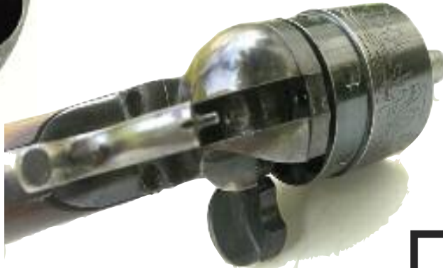
Hole in conversion ring for firing pin, long lip of loading gate
