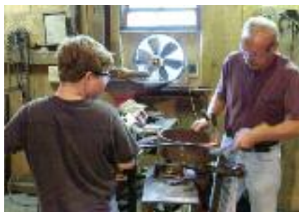
Kyle Loree and Keith Lumbert bending steel. After heating it in the forge they wrapped it around the form and tapped it with a hammer to get the shape they wanted.
